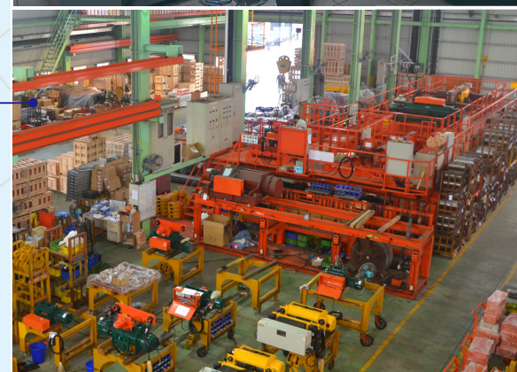
• Wire Rope Hoist Load Test Platform • All Hoist Must Pass 125% Load Test Prior To Shipment
