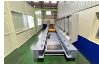
150 ton Horizontal tensile testing machine
