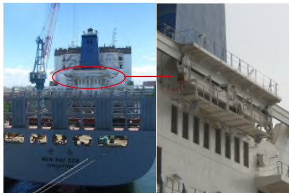
● Provision Crane / Monorail Crane
