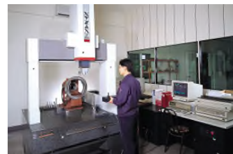
TKS GT 800A 3D Scanning Probe for Highly Precise Measurements
